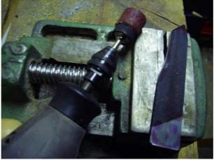
Then, format with the drum of Dremel sandpapering coarse grits (40) to 30 000 tours/mn. I point out that the work of this strongly high-carbon steel will cause very many sparks, protect you to them eyes, the hands and avoid wearing synthetic fiber clothing.
