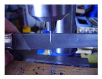
Then, install the point obtained on a drill press (on a drilling machine or Dremel in the chuck that functions too.) Made turn the point at low speed and apply a file very slightly (soft preferably) above in order to reduce very slightly the diameter of the point to be able to introduce it into the holes planned for the tangs.
