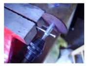
In order to carry out the tang pine, take a nail out of stainless steel of 2.5mm of diameter of which you will cut the head using the disc to cut up Dremel.
