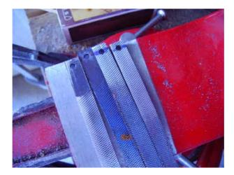
Once the handle with the same width, carry out the holes for the pivots. Mark each branch in its center with the punch,  $(7,5/2=3,75 \,\mathrm{mm}$  of the edge) the 0,75 is done a little with judged because my reglet does not go that at the half mm .On is located at 3,5 mm of the top in order to have 2 mm of margin to make round branches around the axis.
