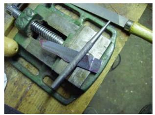
Then, mark the points to be bored for the axes with a punch. The points of drilling are to 1 cm of the heel of the blade and 3,5 mm of each edge for a riveting of 3mm.( which leaves a margin of 2mm of each with dimensions of the pivot.)
