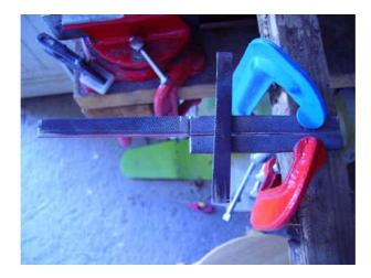
The handle realization is tackled. Once again out of file. As you see it, fixing of the file on a support and then cut in its center with the hacksaw (with a good quality blade one gains enormously in cut cleanliness and time). The handle will make to final 7,5 cm length for 7,5 mm of width.
