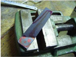
In order to more clearly visualize the profile and the design of the future blade on which one will work, you can trace with the CD marker contours of the blade, as well as the height of the bevel (the line in the center of the file) and materialize the site of the pivots and tangs pins by points. Here to illustrate the matter the blade will have reverse tanto profile.
