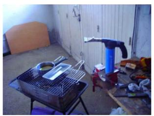
My summary hardening station, a blow lamp, a pan filled with oil of crackling which I heated as a preliminary until the first quivering of oil in order to flux it. One sees a cake mould there filled with water, I confirm that it is not an excellent idea to soak with water this type of steel,
