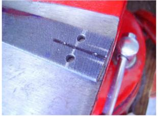
One marks the two tangs pins holes (the nails steels of 2,5 mm slightly improved, put in force and stuck to epoxy in holes of 2 mm). Keep 2 mm of bottom margin, thus mark with 3mm and in the same axis, fix at 3mm top of the pivots to allow the pivots to turn.
