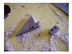
This part is a fall of rasp 4 mm thickness which will use to me to carry out the spacers. These small parts which give the thickness to the sandwich of the handle. These spacers will make all the width of the handle is 7,5mm. Before making drillings, mark with the point a rectangle of 5 mm on 7mm. And, with the punch made two pre holes with 2,5mm of each edge. Drilling will be of 2mm. After that cut the part to the hacksaw.
