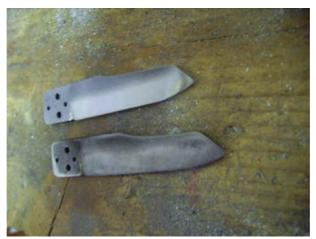
The two blades, that with the crack will be softened, re cut and will finish in "nano bali" and mini spur cutter after being retempered and gone up.
