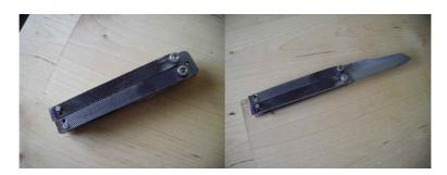
I like to show a first assembly to check the general aspect. I use for that of traditional screws and bolts. On the other hand I carry out an assembly of the parts such as they will be it with the final one, with the washer of each with dimensions of the blade. The tang pines are not assembled yet, therefore not of thrusts.
