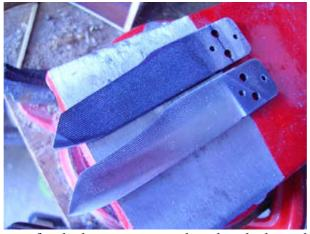
The two blade are ready, on for the heat treatment, the other the have the bevel..
