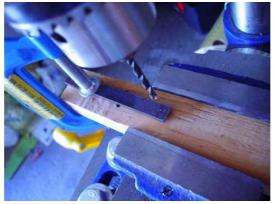
After drilling in 3mm for the axes. (a point that I had forgotten to mention is well to check the perpendicularity of the drill press. Indeed if the unit is slightly inclined, that is likely to obstruct the rotation of the pivots.)
